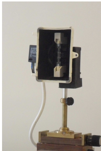
Figure 7. The lamp with linear halogen bulb fixed to an optical bench.
