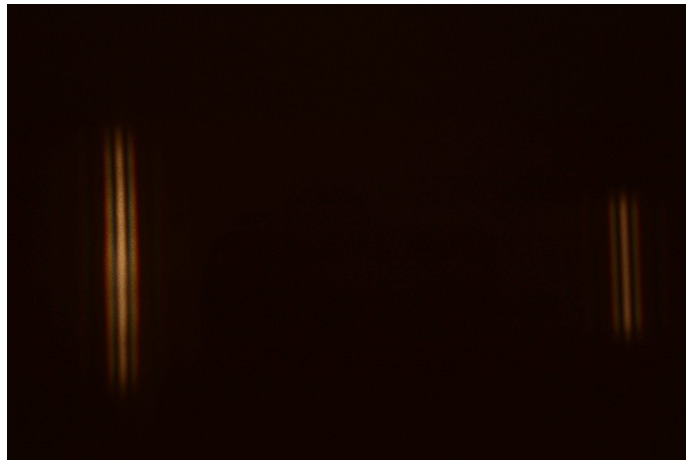
Figure 15. Young diffraction experiment with a single double slit irradiated with linear bulb (left) and 2D bulb (right).
