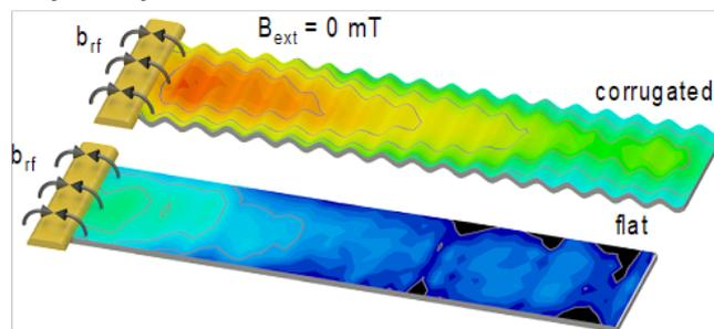
*Spin wave propagation in a waveguide with magnetic anisotropy artificially imprinted perpendicular to the waveguide's long axis (top) compared to a conventional waveguide (bottom).*
