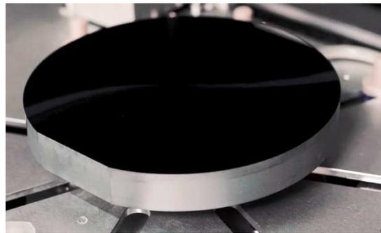
Fig. 2 SiC boule grown by PVT and cut to size
