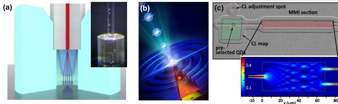
Figure 1: (a) Fiber-coupled QD SPS. (b) Schematic of an electrically controlled QDM device. (c) Integrated quantum circuit realized by in-situ electron beam lithography.
