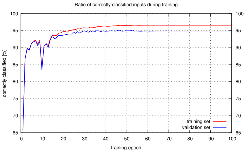
Figure 6.5: Training LeNet-7 architecture ( subs pooling, eta decay) for 100 epochs.
