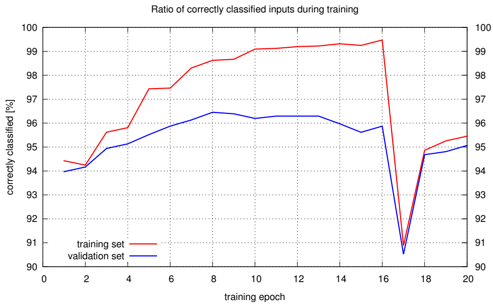
Figure 6.1: Training LeNet-5 architecture ( subs pooling) for 20 epochs.
