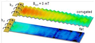
Spin wave propagation in a waveguide with magnetic anisotropy artificially imprinted perpendicular to the waveguide's long axis (top) compared to a conventional waveguide (bottom).
