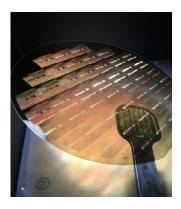
Fig. 4 SiC wafer with devices prior to metallization
