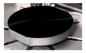
Fig. 2 SiC boule grown by PVT and cut to size
