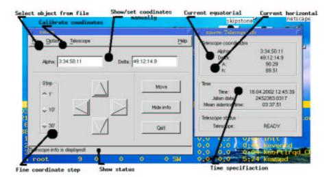
Main window and control panel of xmove. The basic description is included.
