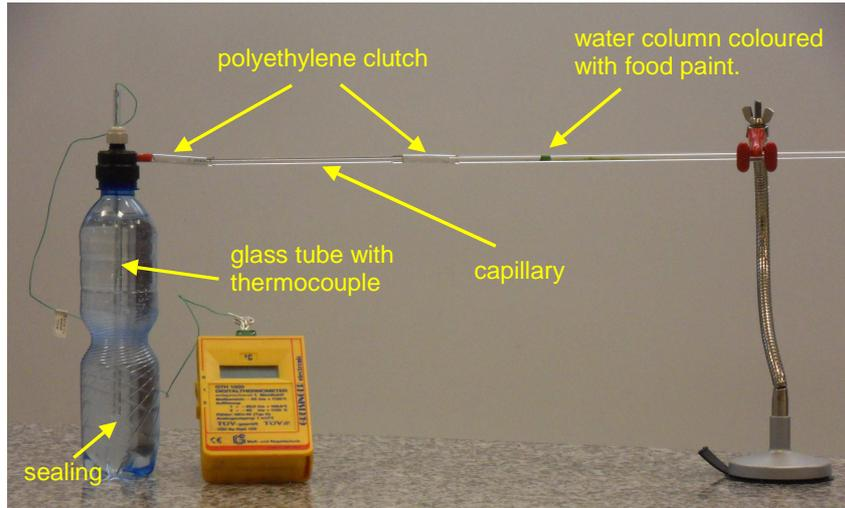
Figure 2: The experimental arrangement.
