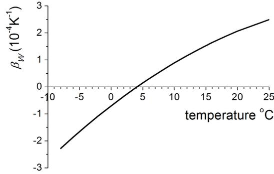
Figure 3: The thermal expansion coefficient of water [3].
