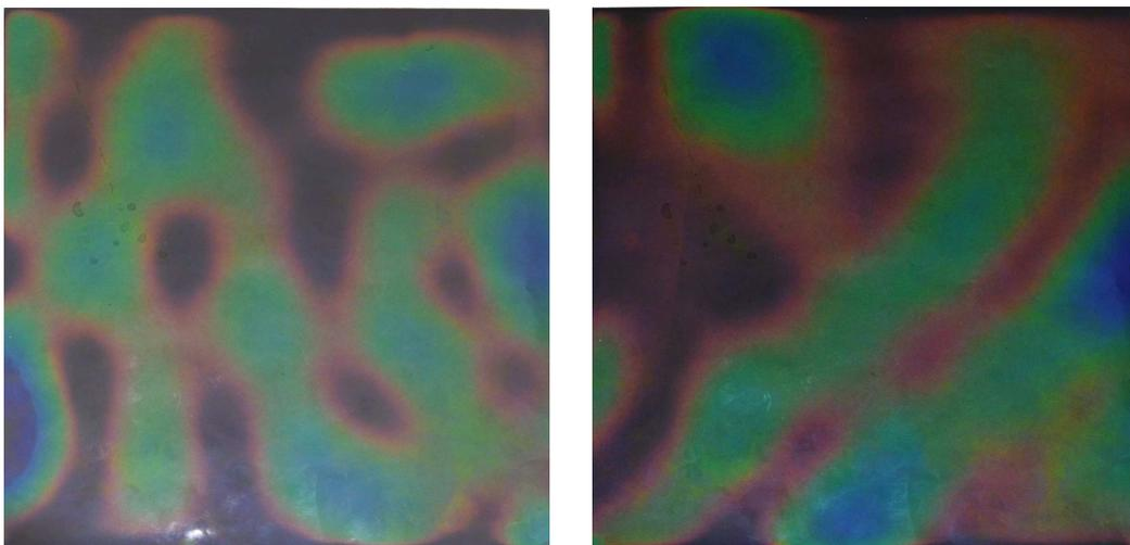
*Figure 5 The examples of the distribution of absorbed microwave power in a MW oven.*
