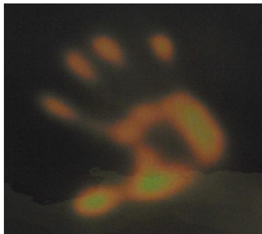
*Figure 1 Heat trace of a human hand.*
