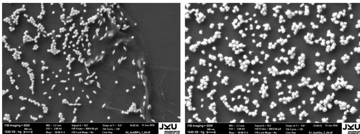
Figure 2: Nanocomposites of graphene with gold bipyramids and nanostars
