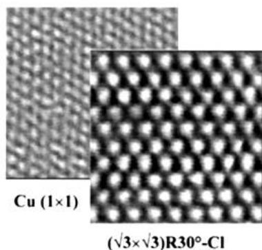
**Figure 2:**  $3.8 \times 3.8 \text{ nm}^2$  EC-STM image of a Cu(111) surface in 10 mM HCl solution with and without Cl- adsorbate [3]
