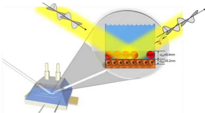
**Figure 1:** Detection of sub-monolayer coverages and the electron excess at electrode surfaces by means of in-situ electrochemical spectroscopic ellipsometry.
