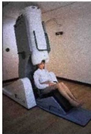
Figure 2: Neuromag Ltd. 122 MEG system
