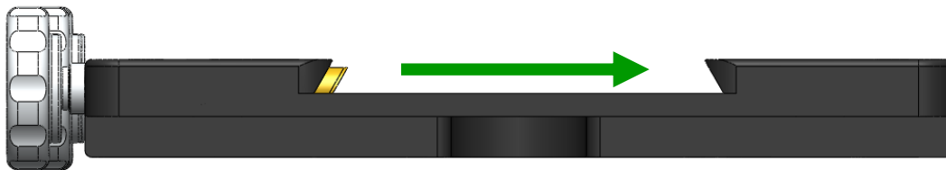
Figure 20: The brass plunger compresses the male dovetail (from left to right in the above diagram).
