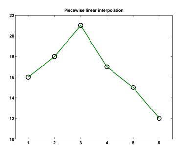
Figure 3.3. Piecewise linear interpolation
