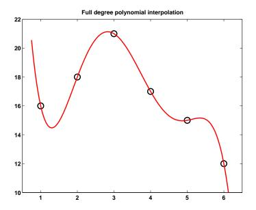
Figure 3.2. Full degree polynomial interpolation
