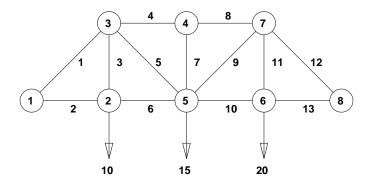
Figure 2.5. A plane truss
