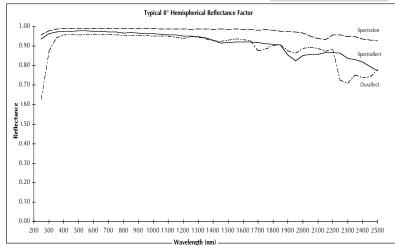
**▼** Typical 8° Hemispherical Reflectance Data Labsphere Infragold Coating
