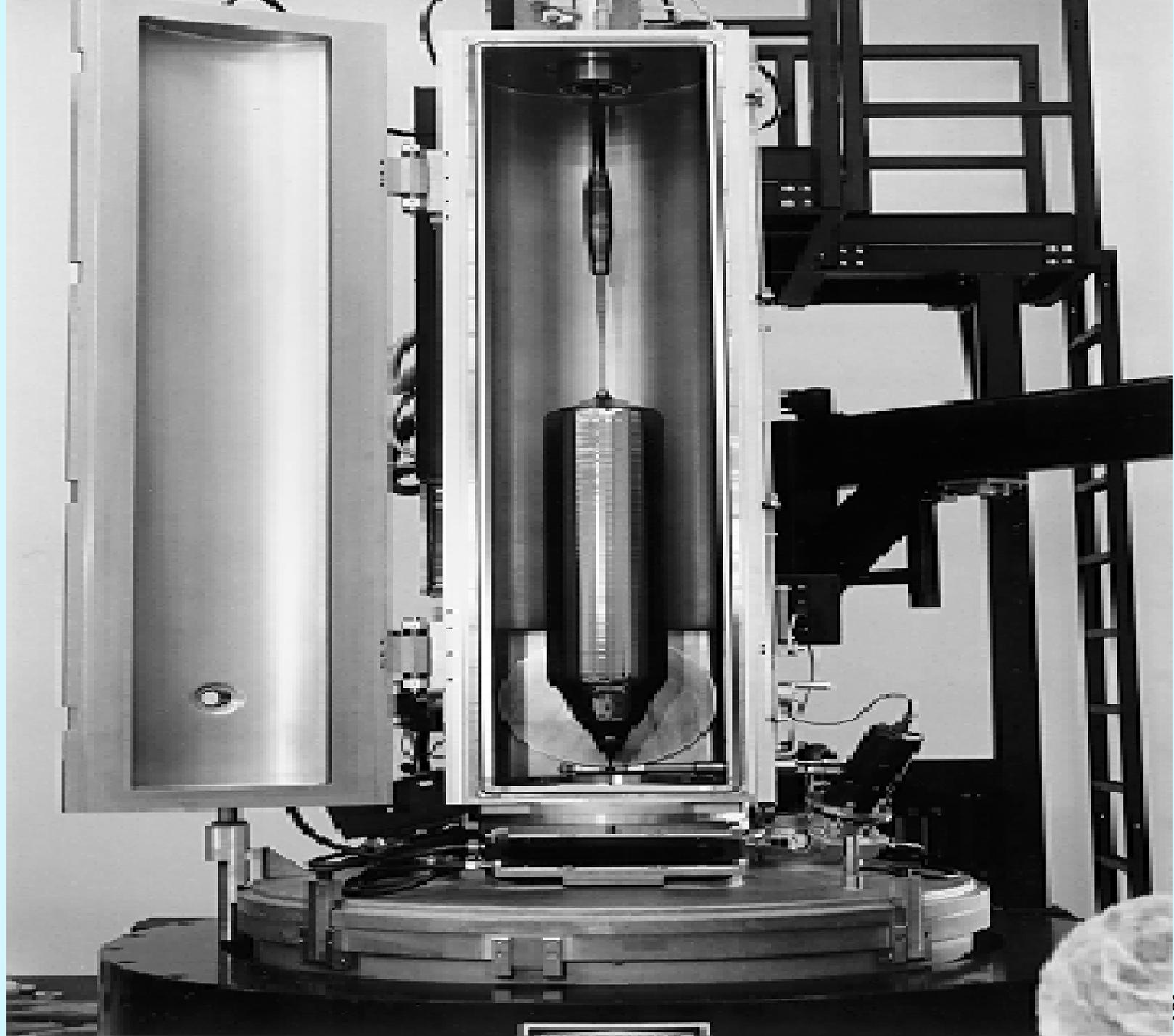
An alternative process is the “**Float Zone**” process which can be used for refining or single crystal growth.
