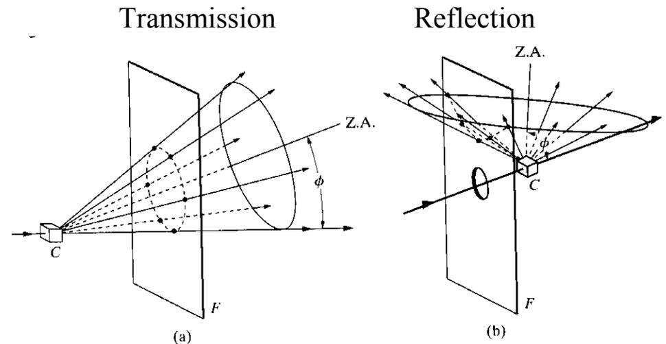
Diffracted beams for reflections in a zone fall on a cone centered around the zone axis
