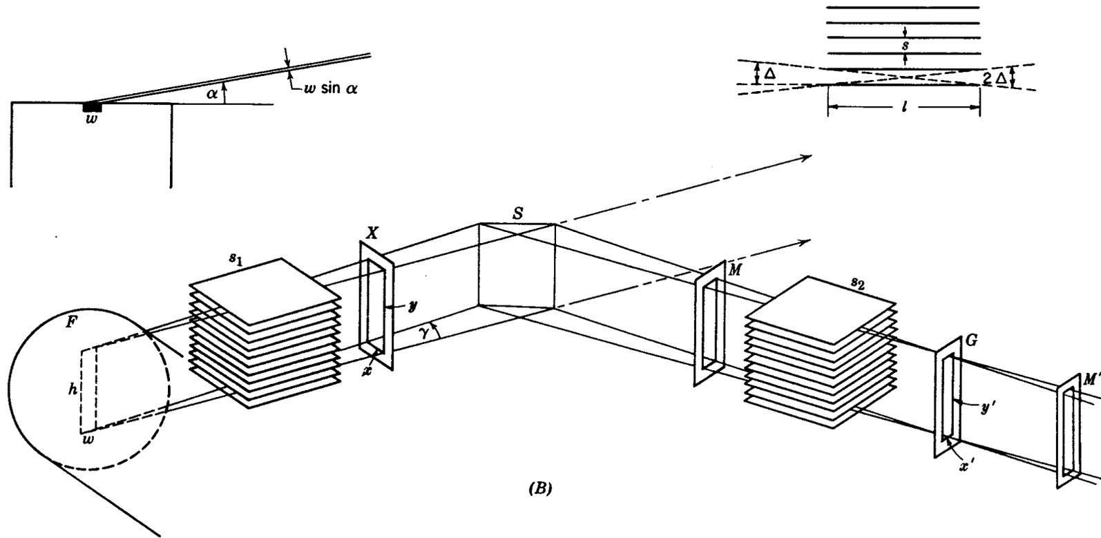
Fig. 5-4. (A) Optical arrangement used in early x-ray diffractometer. (B) Present-day optical arrangement with a "line" x-ray source and Soller slits to limit axial divergence.
