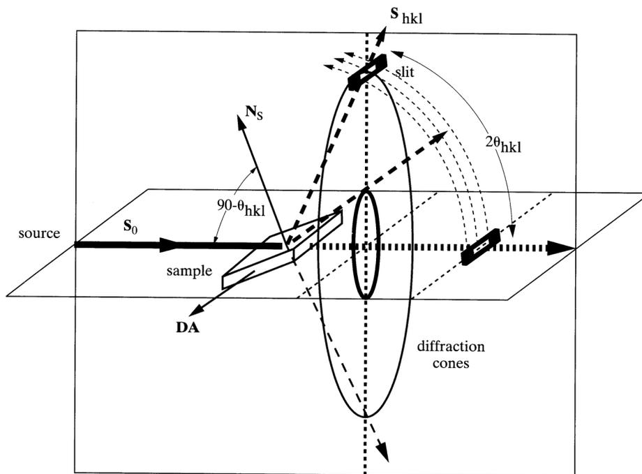
Slit is moved to different  $2\theta$ s. The x-rays passing through the slit are recorded electronically giving a powder pattern
