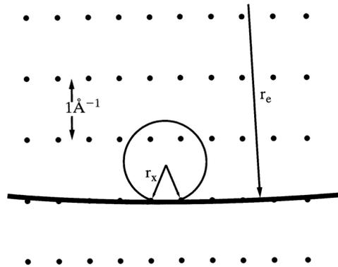
Ewald sphere for Cu radiation is much more curved than that for electrons in an electron diffraction experiment
