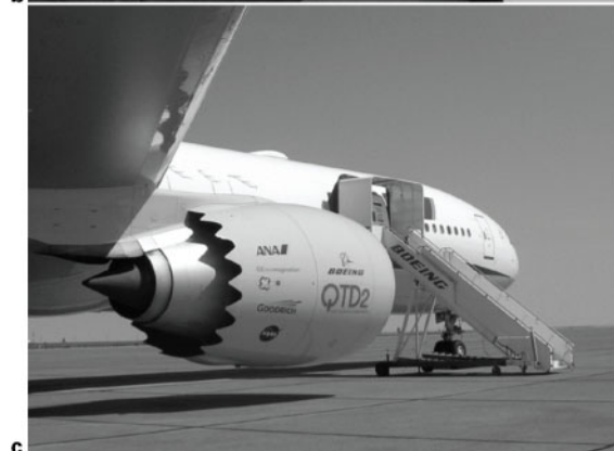
64 Boeing's SMA actuated variable geometry chevron for active or passive noise reduction. a Illustrates the desired configurations of the chevron exhaust nozzle, b SMA bending actuators control the deflection of the chevron and c flight testing of the variable geometry chevron nozzle. 328 Reproduced with permission from the SPIE
