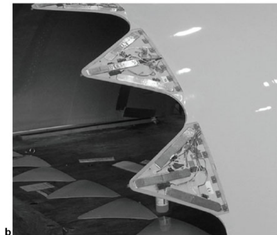
65 Variable geometry nozzle flap design. A system of SMA wires are used to control the configuration of the flap. 332 Reproduced with permission from the SPIE
