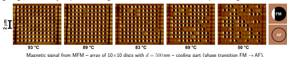
Magnetic signal from MFM – array of  $10 \times 10$  discs with  $d = 500\text{ nm}$  – cooling part (phase transition FM  $\rightarrow$  AF).
