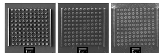
Array of  $10 \times 10$  discs with 500-nm diameter after EBL and negative resist development (left), after IBE (centre) and after BOE etching (right).
