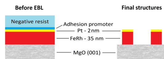
Schema of preparation of FeRh nanostructures.
