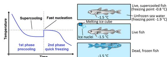
Cooling curve showing the supercooling effect (left). Fish e.g. *Boreogadus saida* (right) survives thanks to the supercooling effect in cold fjord water. Its fluids stay liquid below the freezing point in case of lack of ice nuclei in the environment [6].
