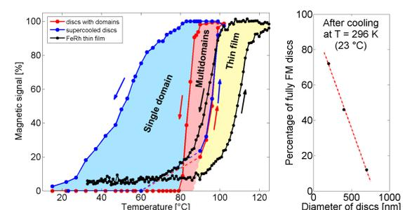
Comparison of averaged magnetic signal (discs, the source thin film, left). Decreasing disc size improving chance to survive supercooled (right).
