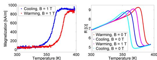
Changes in magnetization and resistivity of a 35-nm FeRh thin film on MgO.
