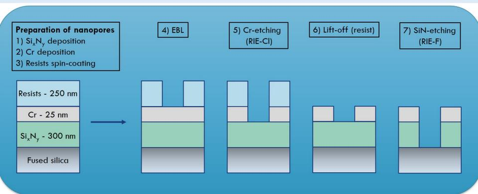
Circular structures with diameter of 50, 100, and 200 nm and variable spacing (300, 500, 1000 nm) were patterned by EBL on MIRA3, TESCAN.
