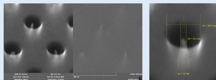
Gold nanomenhirs in 200-nm nanopores (after the mechanical exfoliation).
