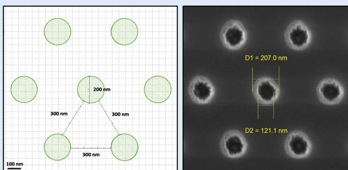
Example of design and final nanopores (circles with diameter of 200 nm, pitch 300 nm).
