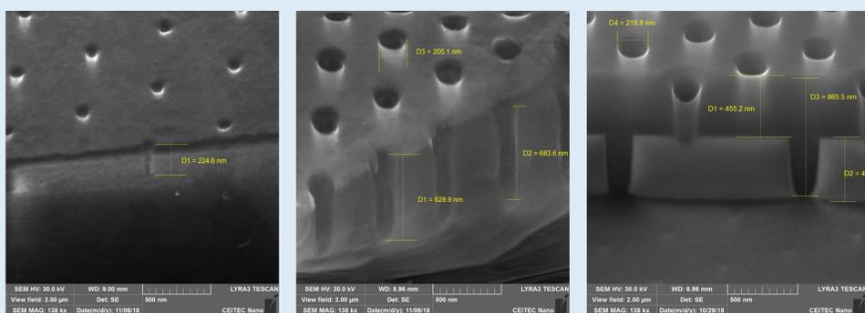
Cross-sections of 100-nm nanopores (pitch 500 nm) and 200-nm nanopores (pitch 300 nm) on the edge of cracks or cut prepared by FIB milling, tilt of 55° (LYRA3, TESCAN).
