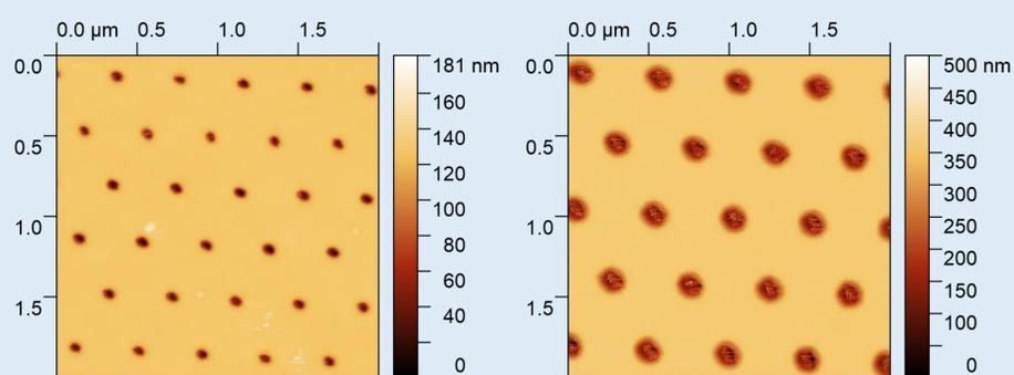
Topography of 100-nm and 200-nm nanopores (pitch 300 nm) using atomic force microscopy technique (DIMENSION ICON, BRUKER).
