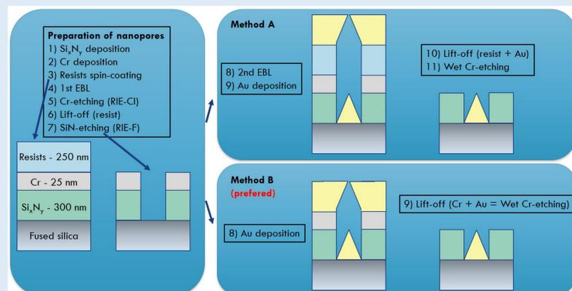
Finding the good deposition properties are the most crucial (rate > 1.5 Å/s [4], tilt 0°, thickness of film similar to depth of pores, E-Beam evaporator).
